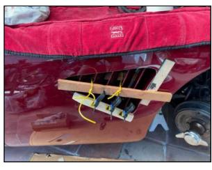
On my first low-speed test without the fan, I was impressed at how warm the left front fender was above the vent. I have not yet enclosed the vent area inside the fender. That implies that the heat was moving out the vent even at city street speeds and without a fan.
