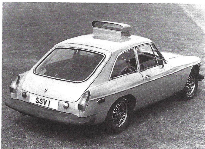
SSV1, with its panoramic mirror, low-soft round nose pedestrian protection bumpers and Dunlop run-flat tyres
