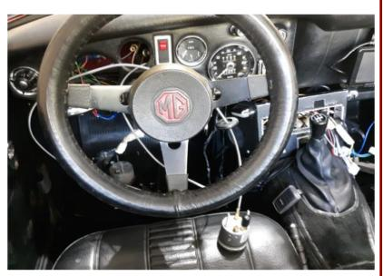
dash just a bit. I just couldn't get enough room for my tubing wrench to fit onto the nut connecting the oil line. I ended up using an old half-inch wrench from a thrift store. But first, I had to grind it a bit thinner and cut a slot in the box end to slip over the oil line.
