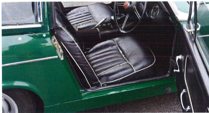
The rear of the front wings is a mud trap where it meets the top of the sill. It's worth checking the sills thoroughly as well
