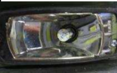
This is a close up view of the latest brake LED (red). Note the lens in the center. It is 60% brighter than the original bulb and consumes only 1/4 of the power.
