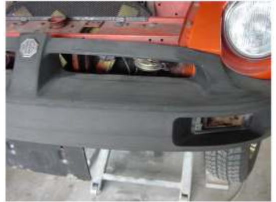
Bumper after cleaning with wax & grease remover
