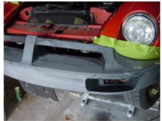
Final sanding before paint
