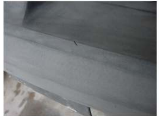
As you can see, a nick like this would stand out on the finished bumper!
